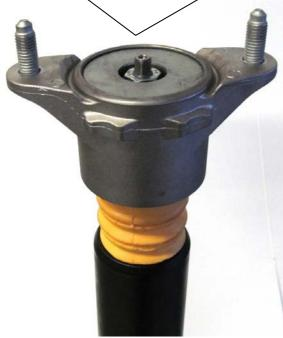
Mount the rear axle adjustment between spring and chassis, the original spring support is no longer used. You have to remove the rear axle adjustment to correct (screw up the threaded ring) the car height.
