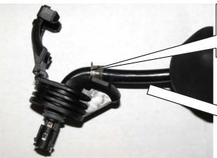
2. Open the connector lock. Remove the Standard wire out of the connector. Use a correct tool.
