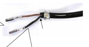
3. Remove the insulation carefully until the metal ring.
