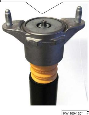
Mount the rear axle adjustment between spring and chassis, the original spring support is no longer used. You have to remove the rear axle adjustment to correct (screw up the threaded ring) the car height.
