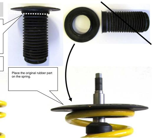
Install the OEM top mount with axial bearing and secure it with the supplied nut. Tightening torque for the piston rod nut is 50 Nm (37 ft-lb). The strut unit has to be installed according to manufacturers recommended settings regarding tightening torque and fixing specifications.
