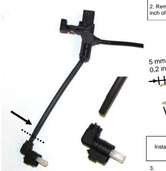
2. Remove 15 mm / 0.6 inch of the cable insulation and 4-5 mm / 0.16 - 0.2inch of the wire insulation. Attach the bend protection.
