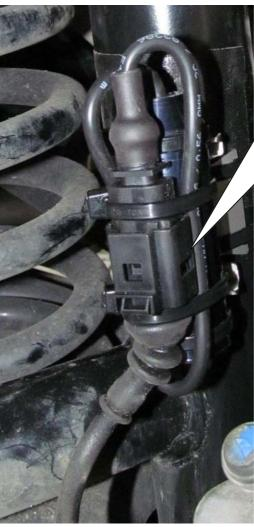
Run the standard damper control wire to the supplied electronic component connector. Insert the standard connector into the electronic component connector until it locks and fix it with cable ties.
