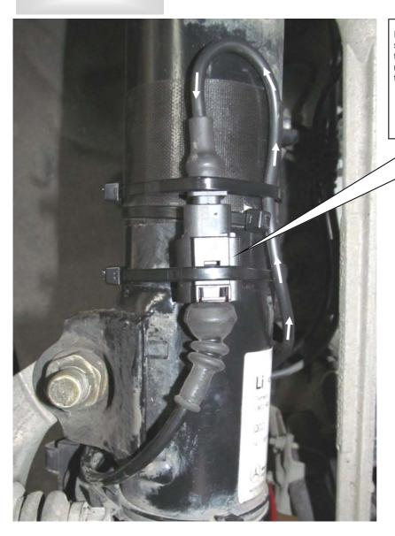
Run the standard damper control wire to the supplied electronic component connector. Insert the standard connector into the electronic component connector until it locks and fix it with cable ties.
