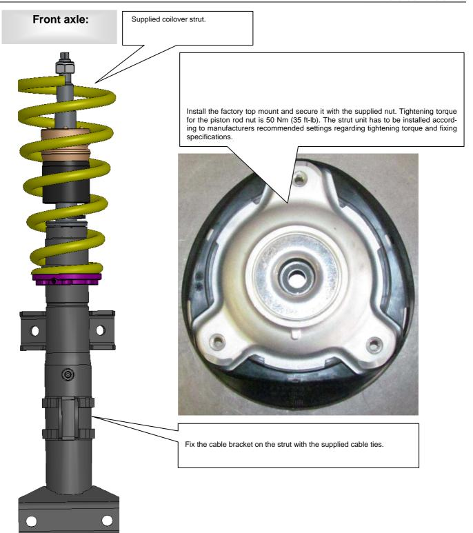
After you have completed installation of the suspension, check the clearance of the tire to the front suspension strut. The minimum clearance at the narrowest point is 5 mm and must, where necessary, be provided using commercially available, Technical Inspectorate (German TUEV) approved spacers.
