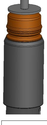
Mount the rear axle adjustment between spring and chassis, the original spring supporting disc is not longer used. You have to remove the rear axle adjustment to correct (screw up the threaded ring) the car height.
