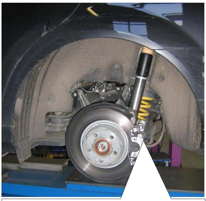
On damper versions with separate reservoirs, mount the reservoir facing the rear of the vehicle as shown on the picture.
