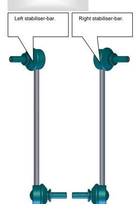
Install the stabiliser-bar as shown on the picture. The stabiliser-bar has to be installed according to manufacturers recommended settings regarding tightening torque. Picture shows left vehicle side.
