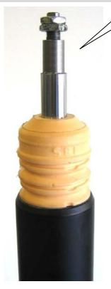
Insert the original supporting bearing and mount it with the supplied nuts. Tightening torque for the piston rod nut is 25 Nm (18ft-lb). The damper unit has to be installed according to manufacturers recommended settings regarding tightening torque and fixing specifications.
