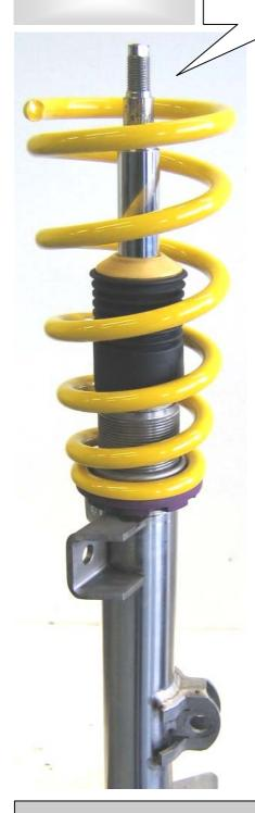
Install the factory supporting bearing and fix it with the supplied stop nut. Tightening torque for the piston rod nut is 50 Nm (37 ft-lb). The strut unit has to be installed according to manufacturers recommended settings regarding tightening torque and fixing specifications.
