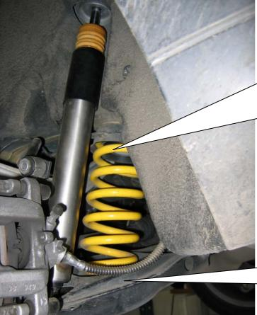
Mount the rear axle adjustment between spring and chassis, the original spring supporting disc is not longer used. You have to remove the rear axle adjustment to correct (screw up the threaded ring) the car height.
