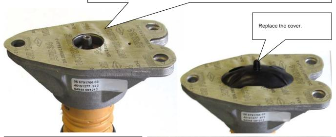
Mount the rear axle adjustment between spring and chassis, the original spring supporting disc is not longer used. You have to remove the rear axle adjustment to correct (screw up the threaded ring) the car height.
