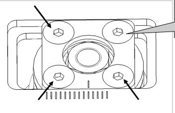
Tightening torque max. 22 Nm (17 ft-lb).
