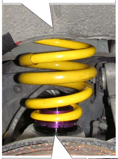
Mount the supplied height adjuster without rubber support between the axle and the lower end of the spring. Remove the original spring perch. Tightening torque is 40 Nm (29ft-lb). Attention: Before the installation of the height adjustment perche the touching surface area have to be cleaned. For the correction of the vehicle height the spring has to be removed.
