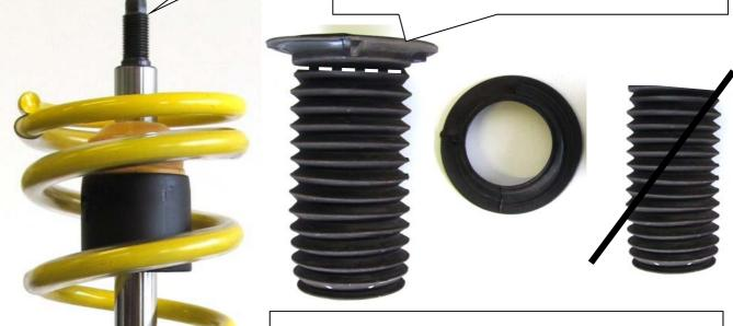
Put the standard supporting bearing unit with spring rubber as shown in the picture and fix it with the supplied nut. Tightening torque for the piston rod is 50 Nm (37 ft-lb). Please install the strut unit to manufacturers recommended settings regarding tightening torque and fixing specifications.
