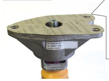
Install the factory top mount and secure it with the standard nut. Tightening torque for the piston rod nut is 50 Nm (37 ft-lb). In addition, the original seal and the cover must be refitted.
