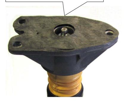
Remove the standard supporting bearing
