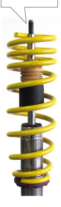
Install the factory top mount and secure it with the supplied nut. Tightening torque for the piston rod nut is 35 Nm (26 ft-lb). The strut unit has to be installed according to manufacturers recommended settings regarding tightening torque and fixing specifications.
