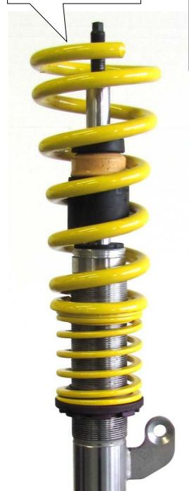
Install the factory top mount and secure it with the supplied nut. Tightening torque for the piston rod nut is 50 Nm (37 ft-lb). The strut unit has to be installed according to manufacturers recommended settings regarding tightening torque and fixing specifications.
