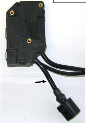
2. Remove 15 mm / 0,6 inch of the cable insulation and 4-5 mm / 0,16 - 0,2 inch of the wire insulation. Attach the heat shrink tube.
