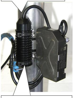
Fix the electronic component on the stainless steel holder with cable ties 4,8mm x 290mm. Additional fix the plug-in connection on the original control box with a cable tie.
