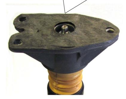
Remove the standard supporting bearing
