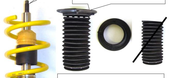
Put the standard supporting bearing unit with spring rubber as shown in the picture and fix it with the supplied nut. Tightening torque for the piston rod is 40 Nm (37 ft-lb). Please install the strut unit to manufacturers recommended settings regarding tightening torque and fixing specifications.
