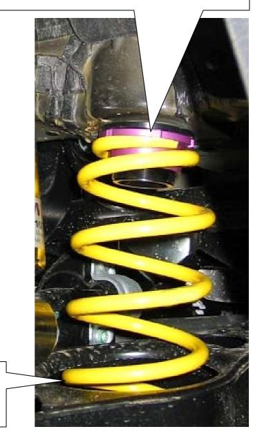
Use the original spring support at the bottom end of the spring.
