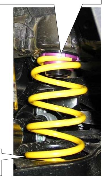
Use the original spring support at the bottom end of the spring.
