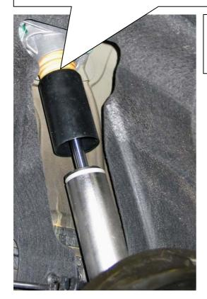
Mount the supplied height adjuster without rubber support between the body and the upper end of the spring.
