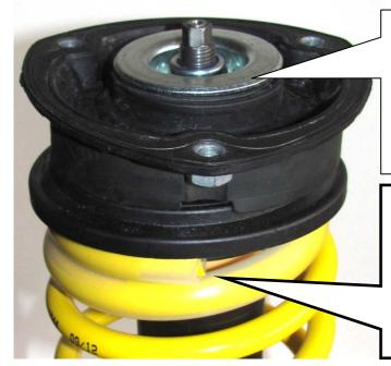
Attach the original top mount and fix it with the supplied nut. Tightening torque for the piston rod is 50 Nm (37 ft-lb). Please install the strut unit to manufacturers recommended settings regarding tightening torque and fixing specifications.
