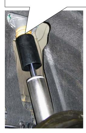
Mount the supplied height adjuster without rubber support between the body and the upper end of the spring.
