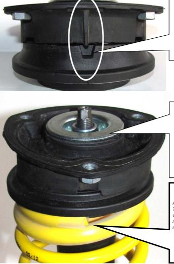
The marks of the OEM upper top mount (upper part) and the OEM axial bearing (bottom part) need to be put on top of each other! The marks show to the vehicle internal side in installed condition.
