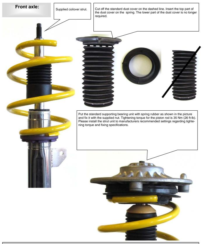
After you have completed installation of the suspension, check the clearance of the tire to the front suspension strut. The minimum clearance at the narrowest point is 5 mm and must, where necessary, be provided using commercially available, Technical Inspectorate (German TUEV) approved spacers.
