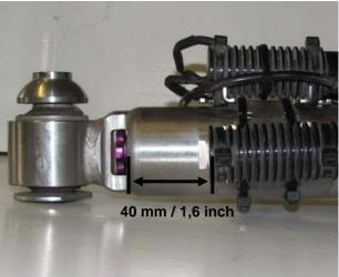
Fix the electronic component on the stainless steel holder with cable ties 4,8mm x 290mm. Additional fix the plug-in connection on the electronic component with a cable tie.
