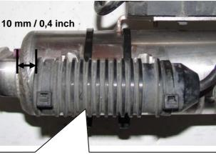
Fix the electronic component on the stainless steel holder with cable ties 4,8mm x 290mm. Additional fix the plug-in connection on the original control box with a cable tie.
