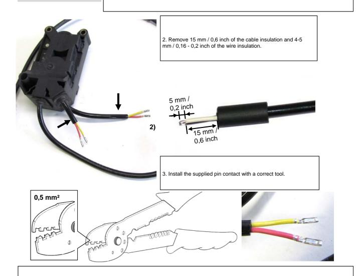
4. Insert the completted wire with sealings into the connector until to the lock. The pinposition / cable colour is not relevant.
