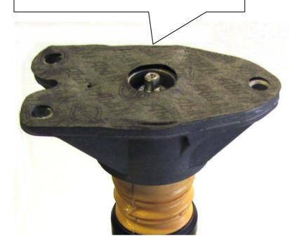
Remove the standard supporting bearing
