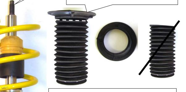
Put the standard supporting bearing unit with spring rubber as shown in the picture and fix it with the supplied nut. Tightening torque for the piston rod is 40 Nm (37 ft-lb). Please install the strut unit to manufacturers recommended settings regarding tightening torque and fixing specifications.
