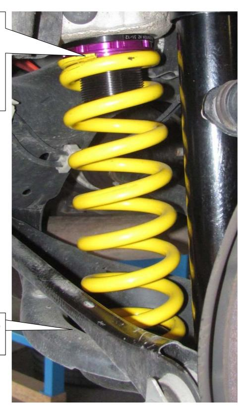
Use the supplied spring adapter at the bottom end of the spring.
