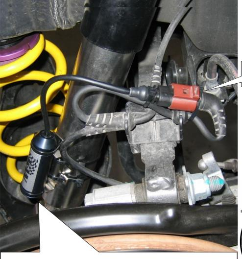
Run the standard damper control and fix it with the small cable ties.
