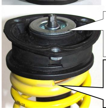
Attach the original top mount and fix it with the supplied nut. Tightening torque for the piston rod is 50 Nm (37 ft-lb). Please install the strut unit to manufacturers recommended settings regarding tightening torque and fixing specifications.
