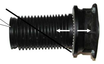
The marks of the OEM upper top mount (upper part) and the OEM axial bearing (bottom part) need to be put on top of each other! The marks show to the vehicle internal side in installed condition.
