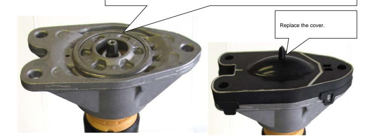
Mount the rear axle adjustment between spring and chassis, the original spring supporting disc is not longer used. You have to remove the rear axle adjustment to correct (screw up the threaded ring) the car height.
