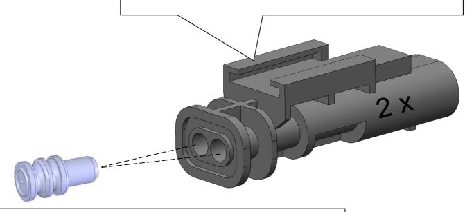
Close the connector  $\,$  of the damper control system with the supplied dummy plug. Fix the connector with cable ties on the wire harness.
