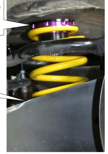
Use the original spring support at the bottom end of the spring.
