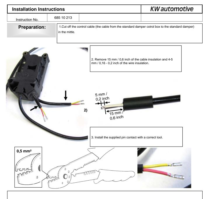
4. Insert the completted wire with sealings into the connector until to the lock. The pinposition / cable colour is not relevant.
