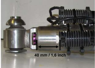
Fix the electronic component on the stainless steel holder with cable ties 4,8mm x 290mm. Additional fix the plug-in connection on the electronic component with a cable tie.
