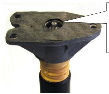
Install the factory top mount and secure it with the supplied nuts. Tightening torque for the piston rod nut is 20 Nm (15 ft-lb). The strut unit has to be installed according to manufacturers instructions settings regarding tightening torque and fixing specifications.
