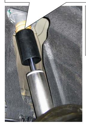
Mount the rear axle adjustment between spring and chassis, the original spring support is no longer used. You have to remove the rear axle adjustment to correct (screw up the threaded ring) the car height.
