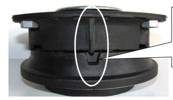
The marks of the OEM upper top mount (upper part) and the OEM axial bearing (bottom part) need to be put on top of each other! The marks show to the vehicle internal side in installed condition.
