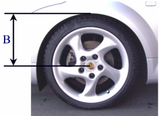
Measurement B Wheel hub center wheel arch
