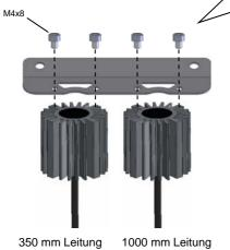
Install the cacellation kit and the holder with the supplied screws and a stopp nut in the ve-
