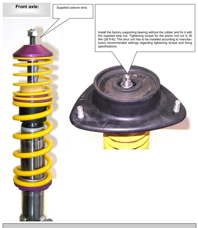
After you have completed installation of the suspension, check the clearance of the tyres to the front suspension strut. The minimum clearance at the narrowest point is 5 mm and must, where necessary, be provided using commercially available, Technical Inspectorate (German TUEV) approved spacers.
