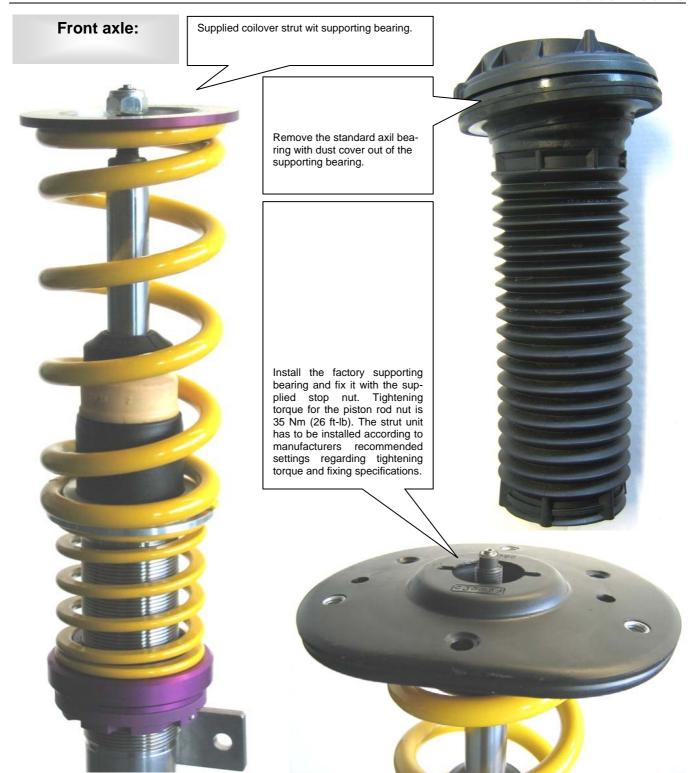
After you have completed installation of the suspension, check the clearance of the tyres to the front suspension strut. The minimum clearance at the narrowest point is 5 mm and must, where necessary, be provided using commercially available, Technical Inspectorate (German TUEV) approved spacers.
