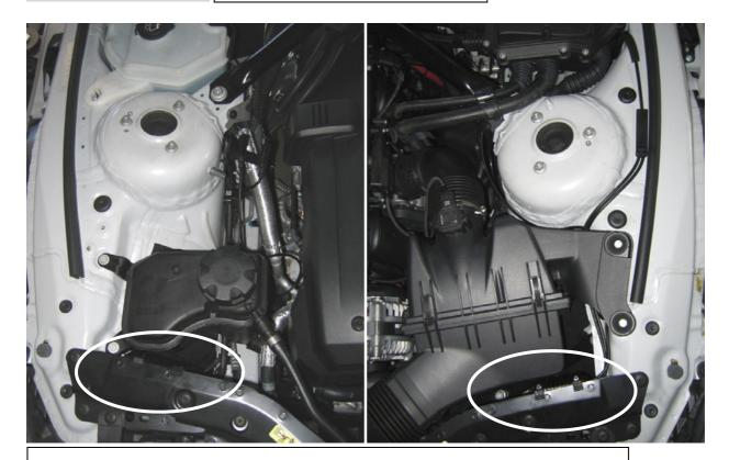
Fix the elektronic component with the supplied edge clips on the front stut.
