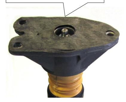
Remove the standard supporting bearing
