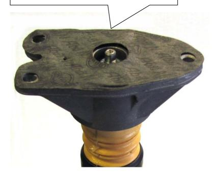
Remove the standard supporting bearing
