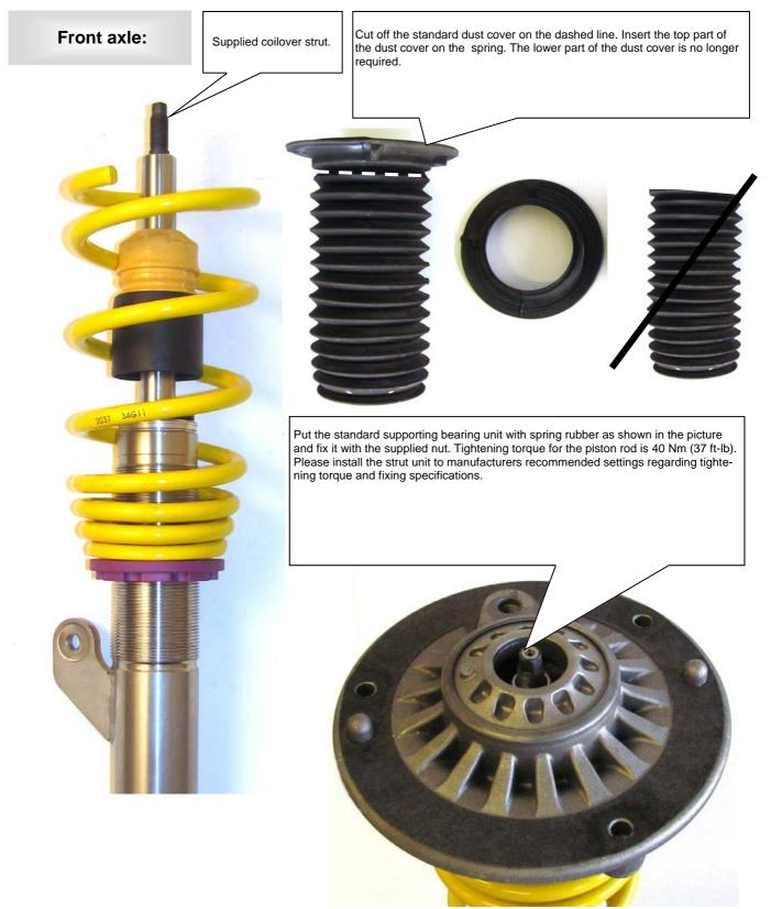
After you have completed installation of the suspension, check the clearance of the tire to the front suspension strut. The minimum clearance at the narrowest point is 5 mm and must, where necessary, be provided using commercially available, Technical Inspectorate (German TUEV) approved spacers.
