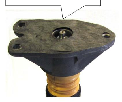
Remove the standard supporting bearing
