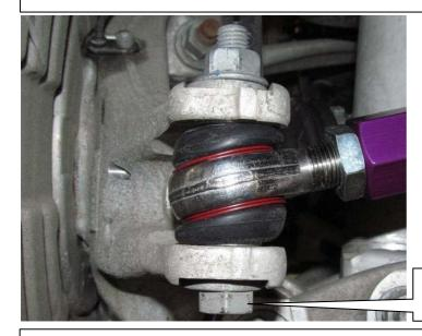
Install original eccentric screw in center position.
