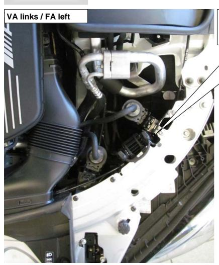
Fix the electronic component with the edge clips on the chassis edge as shown in the picture.
