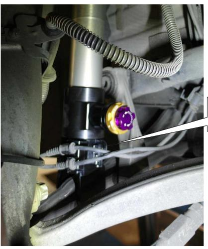
Install the supplied left and right cable bracket on the coilover.
