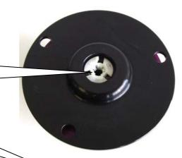
Mount the rear axle adjustment between spring and chassis, the original top spring supporting disc is further used. You have to remove the rear axle adjustment to correct (screw up the threaded ring) the car height.
