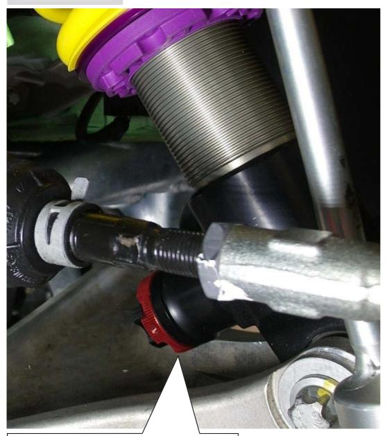
The bump adjustment must shows to the vehicle inside.
