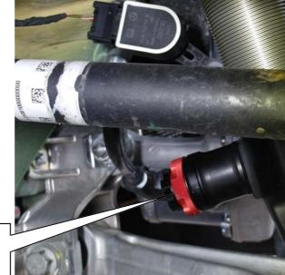
The bump adjustment must shows to the vehicle inside.
