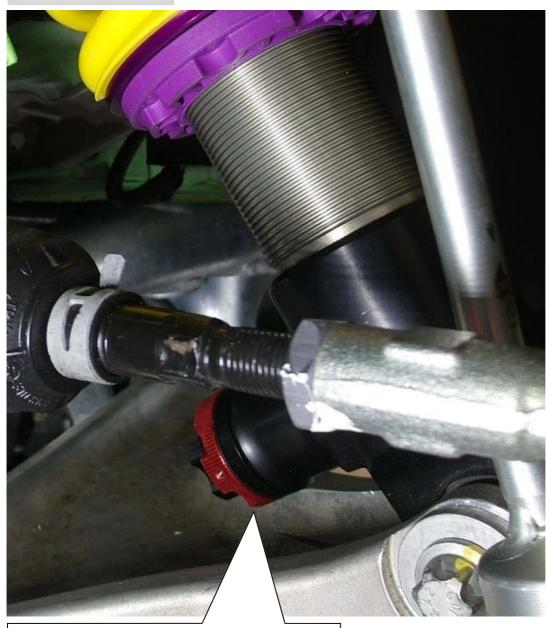
The bump adjustment must shows to the vehicle inside.
