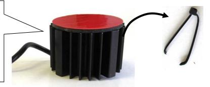
Run the standard damper control wire to the supplied electronic component connector. Insert the standard connector into the electronic component connector until it locks. Fix the canceller with supplied adhesive tape on panel.
