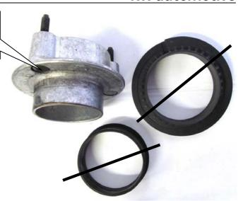
Install the factory supporting bearing and secure it with the supplied nut. Tightening torque for the piston rod nut is 50 Nm (37 ft-lb). The strut unit has to be installed according to manufacturers recommended settings regarding tightening torque and fixing specifications.
