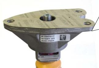
Install the factory top mount and secure it with the standard nut. Tightening torque for the piston rod nut is 50 Nm (37 ft-lb). In addition, the original seal and the cover must be refitted.
