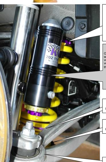
Mount the Mount the rear aear axle adjusxle adjusbtment tment between spring aetween snpring and chassisd chassis,, the original spring supportingthe original spring supporting disc is not longer used.disc is not longer used. YYouou thave to remove have to remove the rearhe rear uaxle adjusted adjustment to correctment to correc
