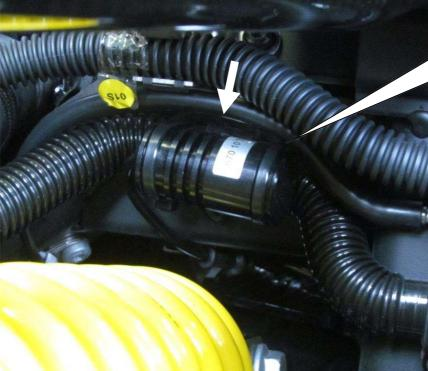
Fix the wire and the connector with cable ties as shown on the picture.
