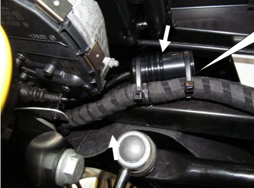
Fix the wire and the connector with cable ties as shown on the picture.
