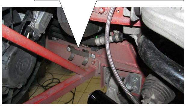
Fix the reservoir with cable ties on the braket. In addition fix the line with cable ties on the wishbone.
