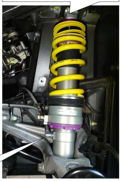
After you have completed installation of the suspension, check the clearance of the tire to the front suspension strut. The minimum clearance at the narrowest point is 5 mm and must, where necessary, be provided using commercially available, technical Inspectorate approved spacers.
