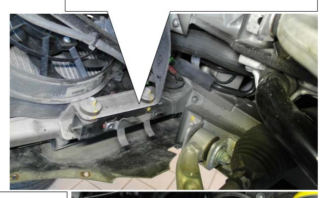
Fix the reservoir with cable ties on the braket. In addition fix the line with cable ties on the wishbone.
