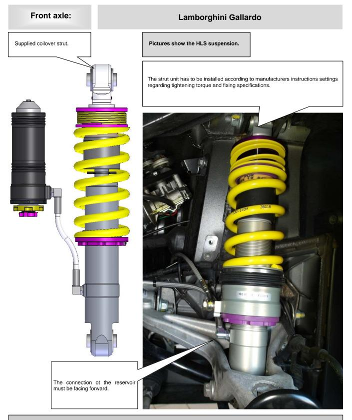
After you have completed installation of the suspension, check the clearance of the tire to the front suspension strut. The minimum clearance at the narrowest point is 5 mm and must, where necessary, be provided using commercially available, technical Inspectorate approved spacers.
