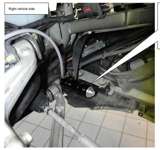
Fix the reservoir with cable ties on the braket. In addition fix the line with cable ties on the wishbone.
