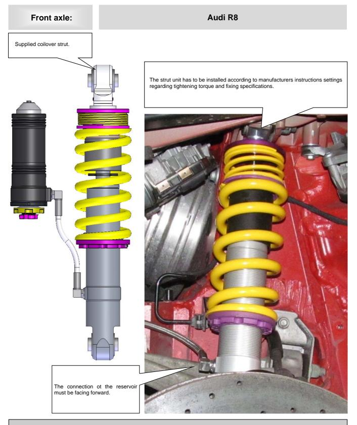
After you have completed installation of the suspension, check the clearance of the tire to the front suspension strut. The minimum clearance at the narrowest point is 5 mm and must, where necessary, be provided using commercially available, Technical Inspectorate approved spacers.
