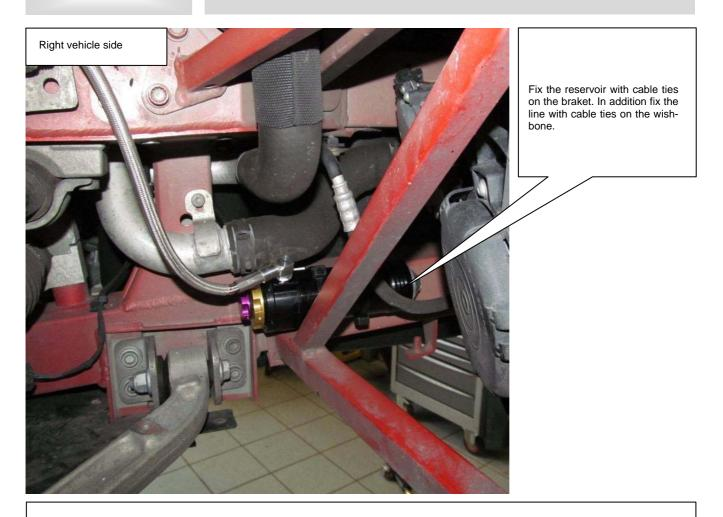
For enough distance between the reservoir and the air conditioning pipe bend the air conditioning pipe to the outside. The conditioning pipe must not touch the reservoir.
