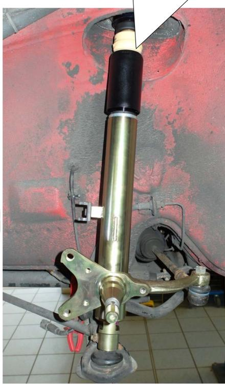
Disassemble the original bearing ring of the OEM strut and mount on new supplied strut. The disassembly and assembly is carried out according to the vehicle manufacturer.
