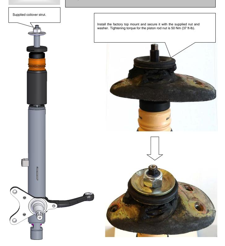
Disassemble the OEM cable holder (if available) from the OEM damper and install it on the supplied damper.
