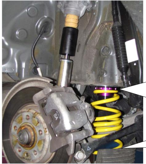
Mount the rear axle adjustment between spring and chassis, the original spring supporting disc is not longer used. You have to remove the rear axle adjustment to correct (screw up the threaded ring) the car height.
