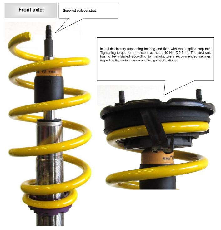
After you have completed installation of the suspension, check the clearance of the tire to the front suspension strut. The minimum clearance at the narrowest point is 5 mm and must, where necessary, be provided using commercially available, Technical Inspectorate approved spacers.
