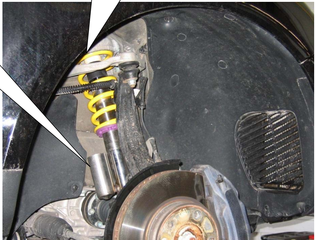
Assembled coilover strut in the car.
