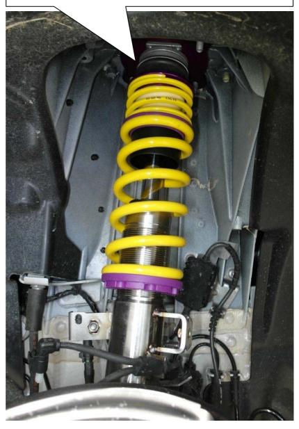
After you have completed installation of the suspension, check the clearance of the tire to the front suspension strut. The minimum clearance at the narrowest point is 5 mm and must, where necessary, be provided using commercially available, Technical Inspectorate approved spacers.
