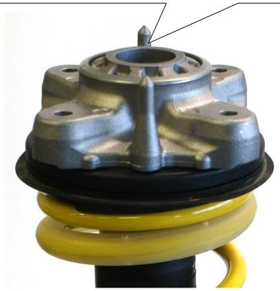
Partial for different vehicle models there are mounted oem vibration absorbers on the coilover struts. Mount this again on the new shock absorber
