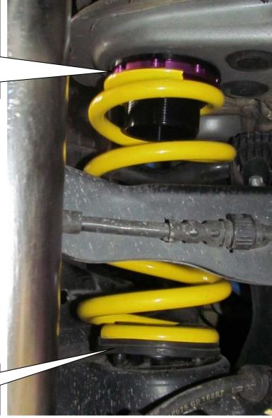
Use the original spring support at the bottom end of the spring.
