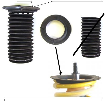
Put the standard supporting bearing unit with spring rubber as shown in the picture and fix it with the supplied nut. Tightening torque for the piston rod is 40 Nm (29 ft-lb). Please install the strut unit to manufacturers recommended settings regarding tightening torque and fixing specifications.
