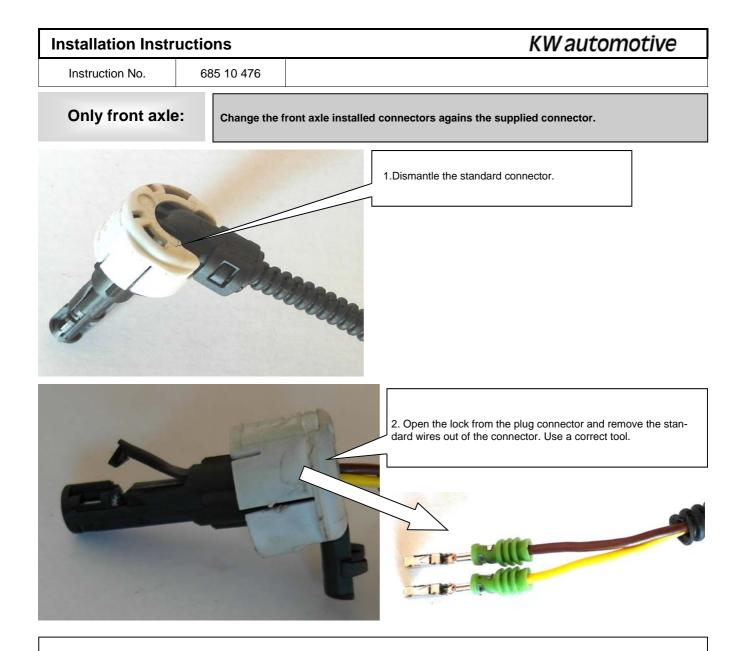
3. Insert the wire completted into the supplied connector until to the lock. The pinposition / cable colour is not relevant. Subsequently lock the connector.
